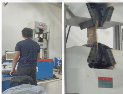
Fig 4. Geotextile tested in ASTM D4632
