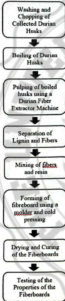
Fig. 3. Durian fiberboard manufacturing process
