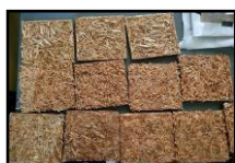
Figure 21. Talahib grass with Polyester resin particle board samples before Modulus of Elasticity tests
