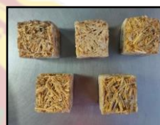
Figure 19. Talahib grass with Polyester resin particle board cube samples after compression test
