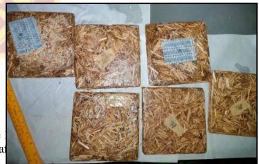
Figure 11. Talahib grass with Polyester resin particle board before submerging in water
