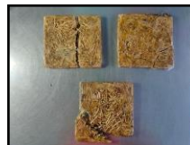
Figure 22. Talahib grass with Polyester resin particle board samples after Modulus of Elasticity tests
