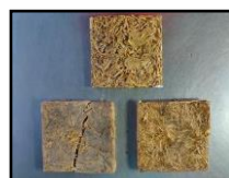
Figure 23 Talahib grass with Polyester resin particle board samples after Modulus of Elasticity tests
