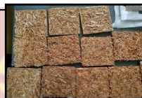
Figure 15. Talahib grass with Polyester resin particle board before the flammability test
