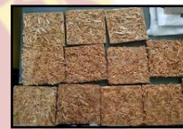
Figure 11. Talahib grass with Polyester resin particle board before submerging in water
